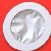
Baader filter material in homemade holder
